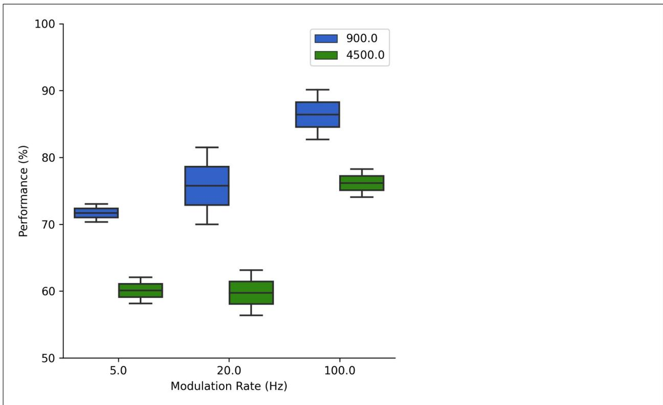
Figure 5.5 Pulse ITD performance for each modulation rate. Performance measured as percentage correct according to pulse ITD stimulus. Data for 900 pps shown in blue and for 4500 pps in green. Boxes indicate mean and interquartile range. Box whiskers indicate 99 % confidence intervals determine from bootstrap method. Repetition rates are pooled together.
