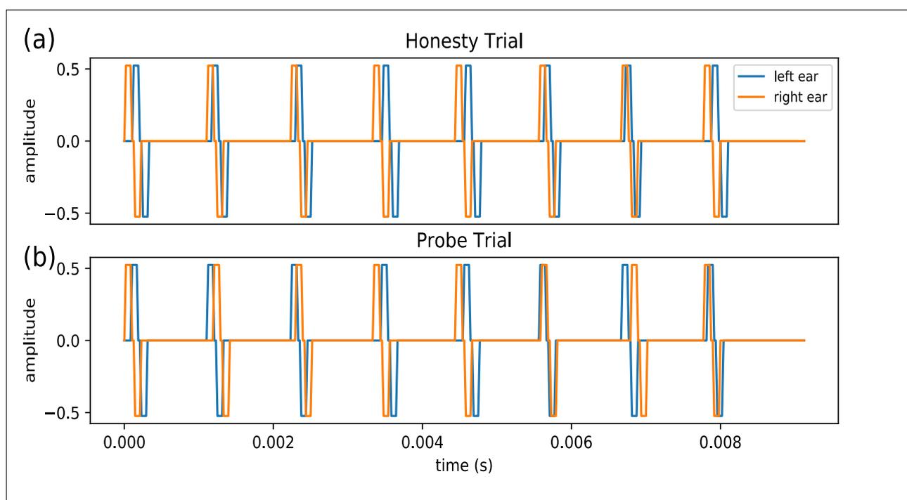
Figure 4.1 CI jittered ITD stimulus example. Right ear stimuli are shown in orange and blue indicates left pulse trains. (a) Example of honesty trial with all pulses consisting of ITDs pointing towards the right (orange pulses). (b) Example of probe trial with ITDs point both left (blue) and right (orange).
