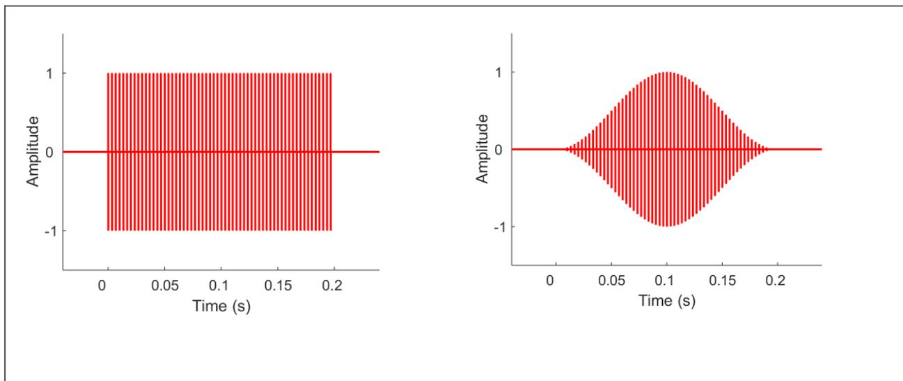
**Figure 3.2 Representative electrical stimuli for rectangular windowed stimulation (left) and Hanning windowed stimulation (right).** Example waveforms of 200 ms duration are shown for a pulse rate of 300 pps.
