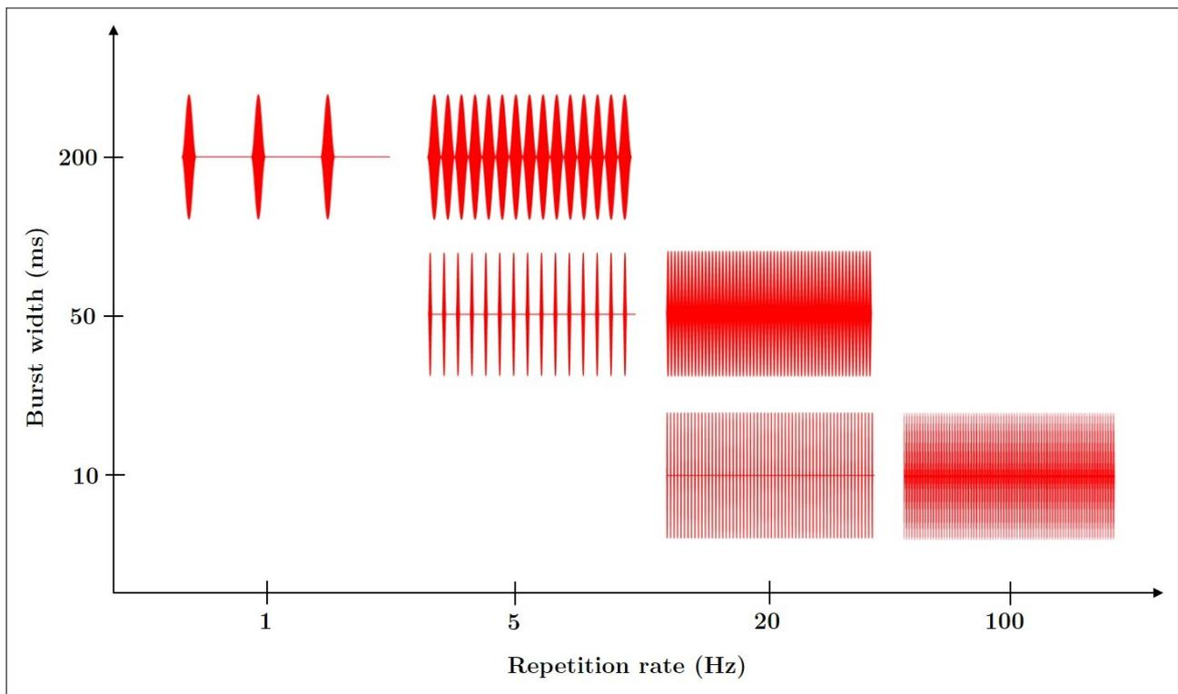
Figure 5.2: Stimulus envelope shapes. Burst width (y-axis) and repetition rate (x-axis) were both varied. Each stimulus has a duration of 3 s. Only the envelope shapes are shown, no individual pulses. The number of pulses in each burst depended on the carrier rate (900 or 4500 pps).
