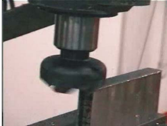
Fig. 5-5. Snapshot of milling head with cBND coated WC and uncoated WC cutting inserts under ball milling test.
