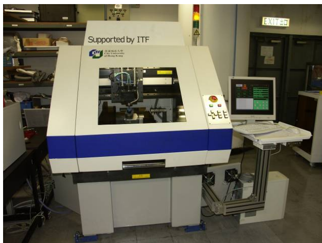
Figure 5.1 Outlook of the homemade 5-axis CNC machine
