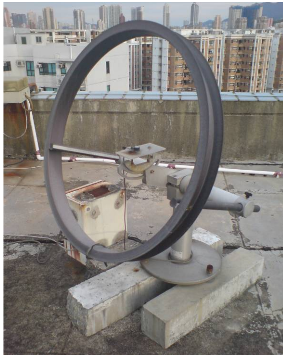
Figure 2.4 Illuminance sensor fitted with shadow ring used for horizontal diffuse illuminance measurement
