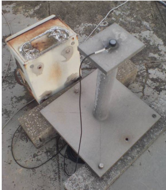
Figure 2.3 Illuminance sensor used for horizontal global illuminance measurement
