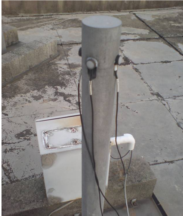
Figure 2.5 Illuminance sensors used for vertical global illuminance measurement
