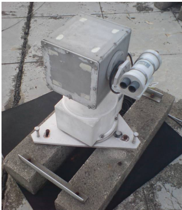
Figure 2.6 Sky scanner used for sky luminance distribution measurement
