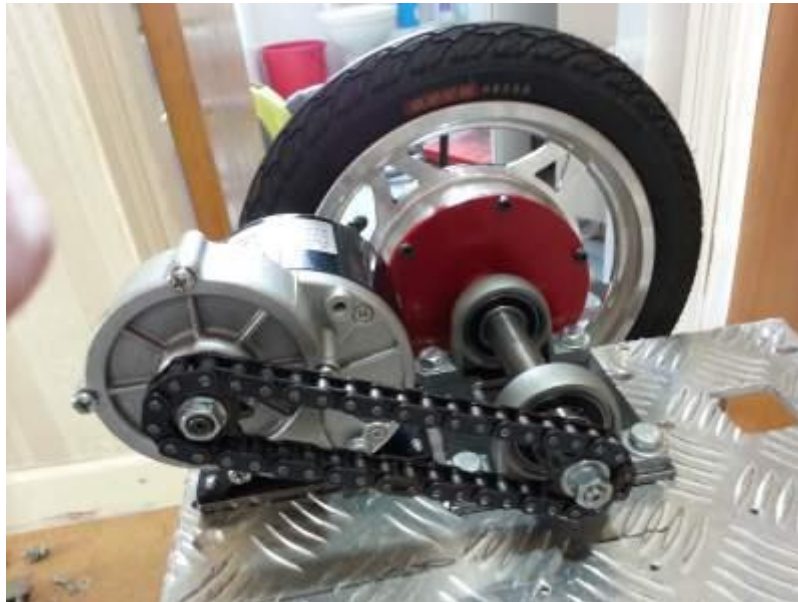
Figure 32: Motor and Wheel connected with a chain mechanism
