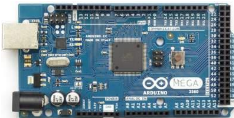
Figure 15: Arduino Mega2560 controller board
