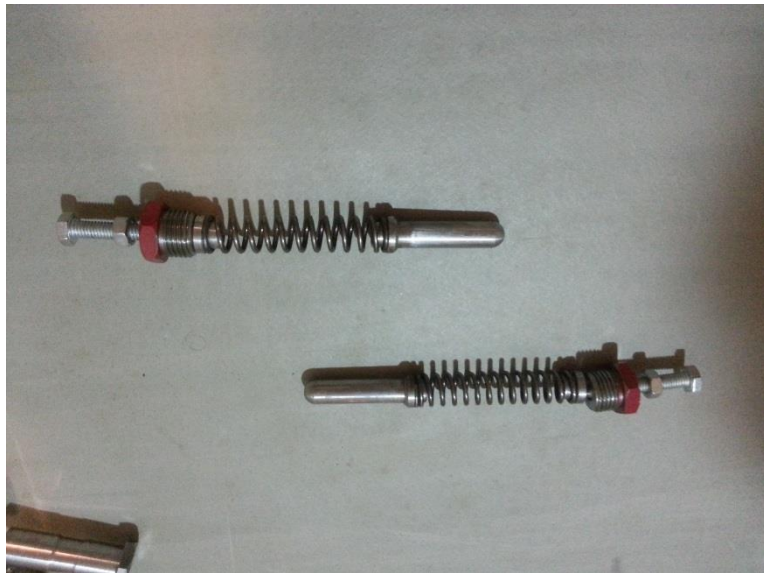
Figure 38: Springs used in the handlebar case
