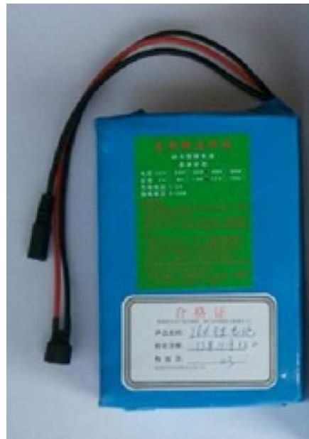
Figure 12: A Lithium Iron Phosphate battery
