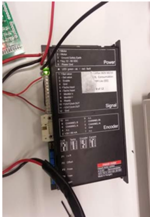
Figure 14: Maxon motor controller board
