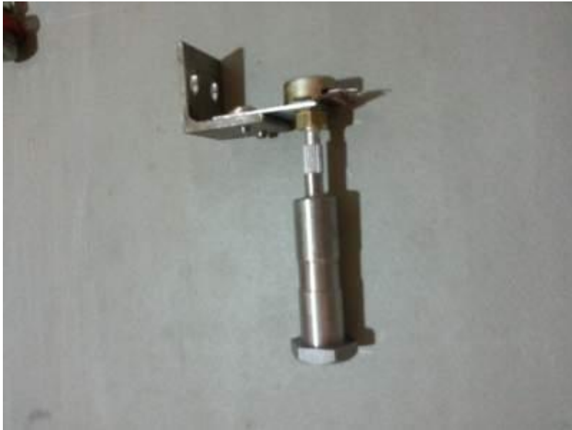
Figure 37: Connection part, base and the variable resistor
