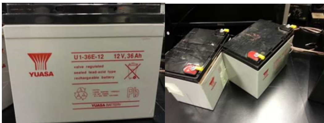
Figure 11: Detail of a lead–acid battery
