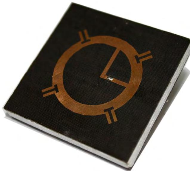
*Fig.5.1.1 (c) 3D view of second prototyped proposed antenna*
