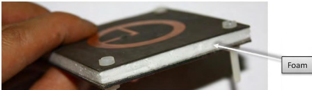
Fig. 4.2 (e) Slant view of fabricated first proposed antenna
