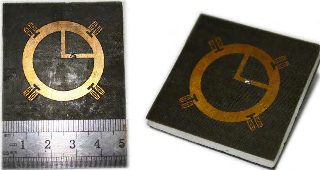
*Fig.5.2.1 (b) Top and 3D view of third prototyped proposed antenna*
