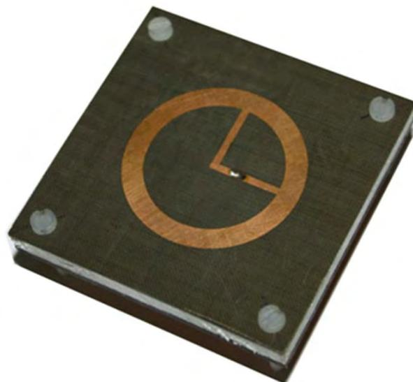
Fig. 4.2 (f) 3D view of fabricated first proposed antenna
