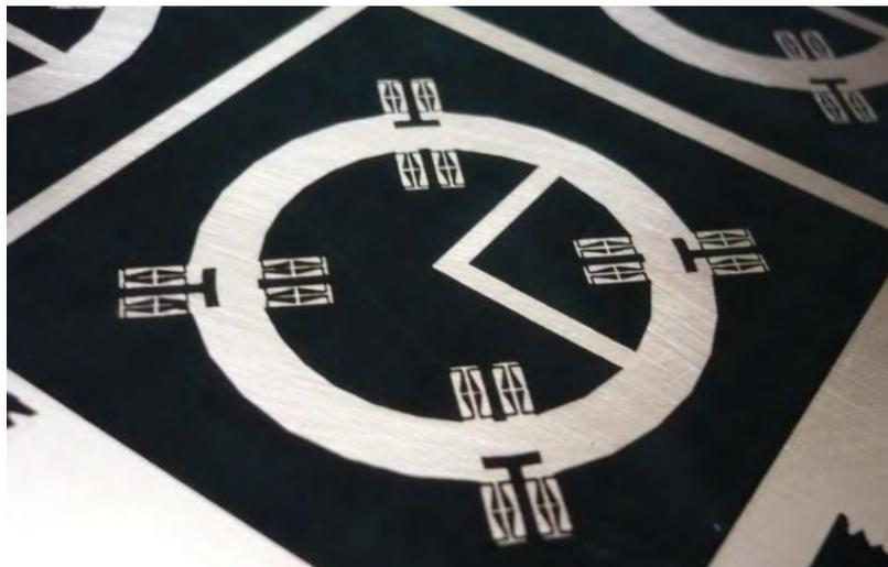
*Fig. 5.2.1 (a) Prototype of fourth proposed antenna*
