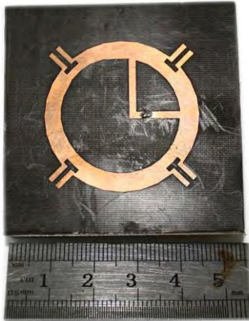
*Fig.5.1.1 (b) Top view of second prototyped proposed antenna*
