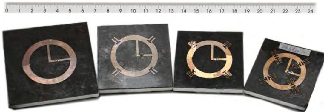
*Fig.5.4 (a) Prototype of 1<sup>st</sup> to 4<sup>th</sup> proposed antenna*
