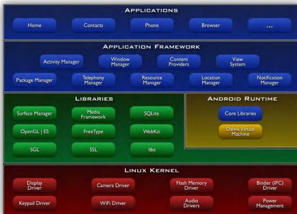
Figure 2.3.2.1a: Major components of Android™ operating system
